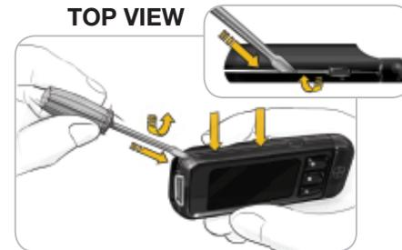
Pry up rechargeable battery here (A). Disconnect battery by pulling battery connector (B).
