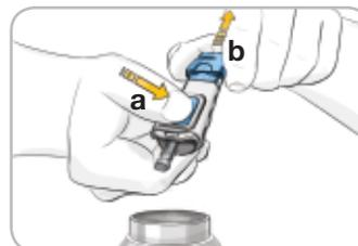
4. While pressing the release button (a), pull the re-setting handle (b), and the lancet will drop into the container you have selected.
