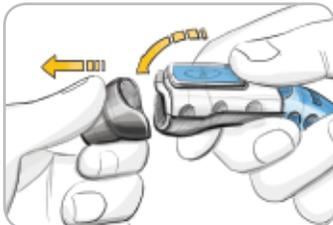
1. To remove the endcap, hold the device with your thumb on the grip indent and hold the endcap dial in the other hand. Snap the endcap off from top to bottom.
