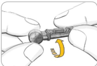
2. Loosen the round protective cap on a lancet by rotating it 1/4 turn, but do not remove it.
