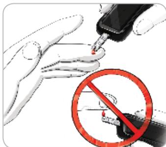
4. Immediately touch the tip of the test strip in the blood drop until the meter beeps. The blood is pulled into the test strip through the tip.
