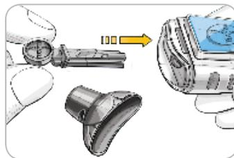
3. Insert the lancet firmly into the lancing device until it comes to a full stop. This will re-set the device. You can also pull and release the re-setting handle.
