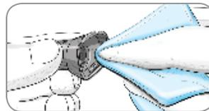
3. Using a new Clorox Germicidal Wipe, carefully wipe all external and internal surfaces of the endcap until wet.
