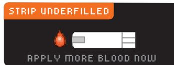
Follow the instructions on the meter screen. If you do not apply more blood within about 30 seconds, remove the strip and start over with a new strip.
