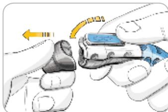
1. Remove the endcap from the MICROLET®2 lancing device with your thumb on the grip indent as shown. Snap the endcap off from top to bottom.
