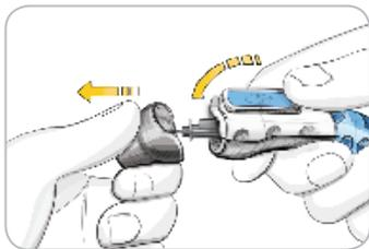
1. In one hand, hold the lancet device with your thumb on the grip indent, with your other hand, hold the endcap as shown, and gently snap off the endcap.
