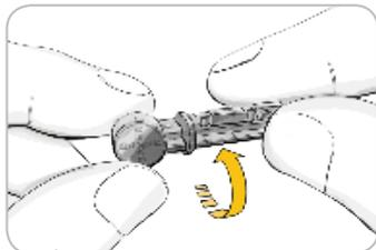
2. Loosen the round protective cap on a lancet by rotating it  $\frac{1}{4}$  turn, but do not remove it.
